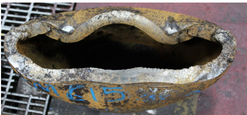
14.15" Q-125 127# casing after WBSR-X shear
