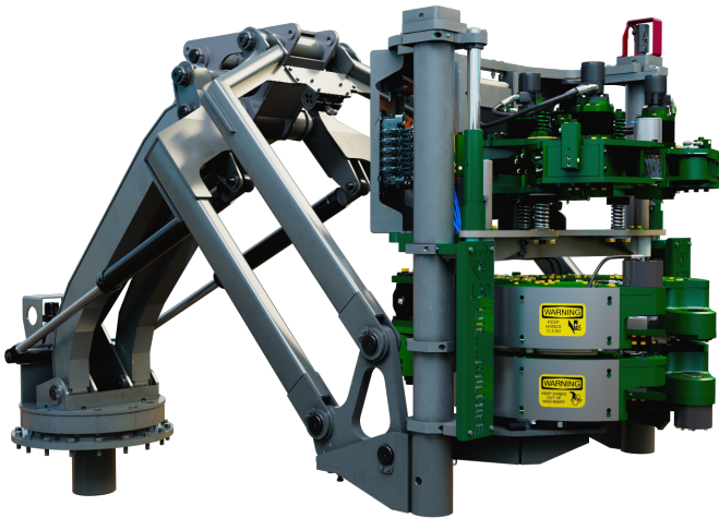
360° radial contact provides evenly applied pressure to the pipe.
