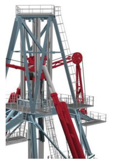
HMH drillstring compensator keeps the vertical force virtually constant
