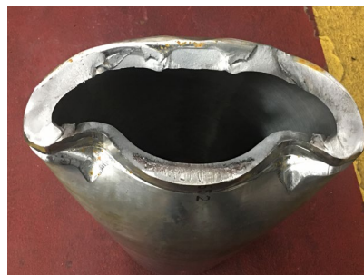
10.75IN. 108.7 lb/ft, SDSS/125KSI casing after WCSR-X shear
