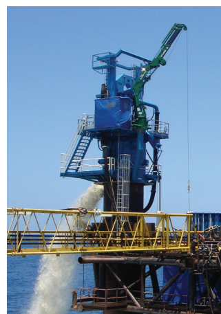
Australia – North West Shelf PBA 936/3000/300 for foundation of the Angel oil and gas platform. Drilling diameter of 3.0 m and a drill string length of up to 110 m
