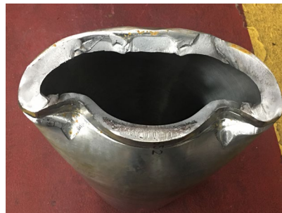
10.75IN. 108.7 lb/ft, SDSS/125KSI casing after WCSR-X shear
