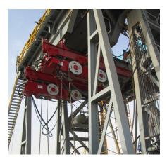
Our design with mono-rail track provides smooth carriage travel, better visibility, and greater freedom of movement. Adjustable from 20 to 50 ft above drill floor
